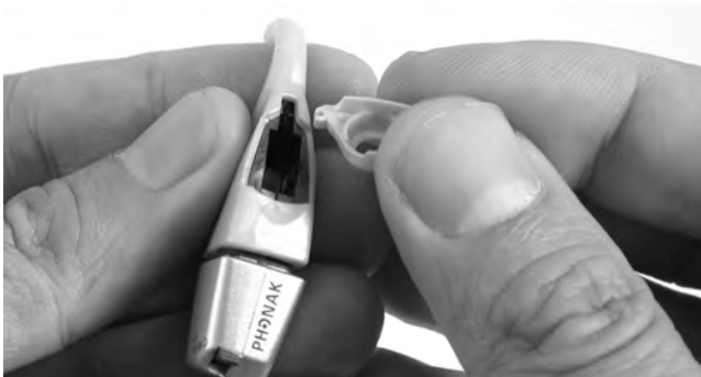
Figure 30: Installing a New Battery Compartment.
