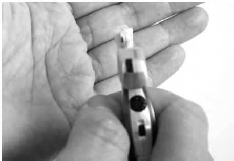
Figure 28: Removing Old Battery.
